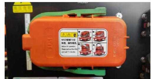
The electrical system is equipped with high-voltage interlocks, insulation detection, offering vehicle-grade safety measures. The MSD maintenance switch enables one-click power-down and safer maintenance;
