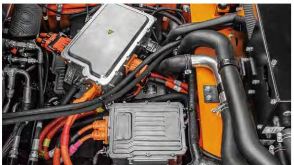
Both the drive and operating systems are vehicle-grade permanent magnet synchronization systems. Equipped with a high speed ratio gearbox, the driving speed, lifting speed, upslope degree and acceleration performance surpass that of internal combustion vehicles.
