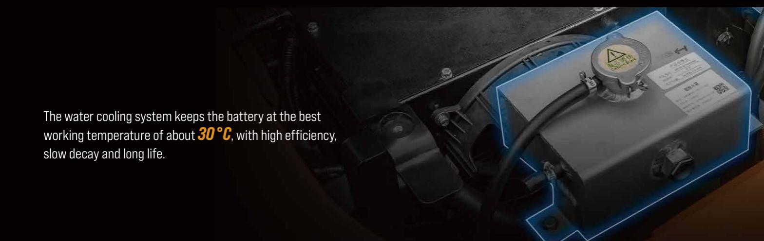
The water cooling system keeps the battery at the best working temperature of about **30 °C**, with high efficiency, slow decay and long life.
