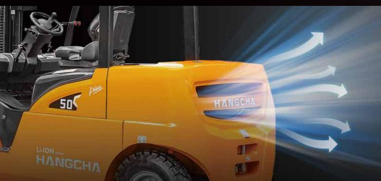
The **large ventilation opening** designed for internal combustion forklifts allows better heat dissipation of the battery and the motor.
