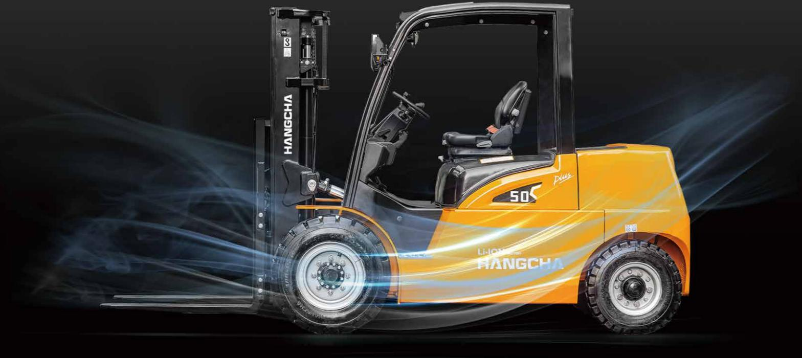
*It is the first time that the motor-battery dual water cooling systems and full suspension damping system are used on new energy forklifts, which can be fully applicable to various severe operating conditions such as high temperature and strong load.*
